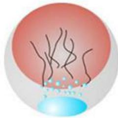
After steam heating, the raw material pentane of EPS begins to boil ⇒ EPS beads began to expand.
